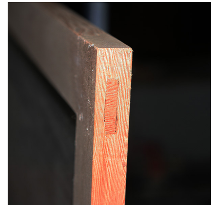
Fig. 1 Through-mortise and tenon joint
